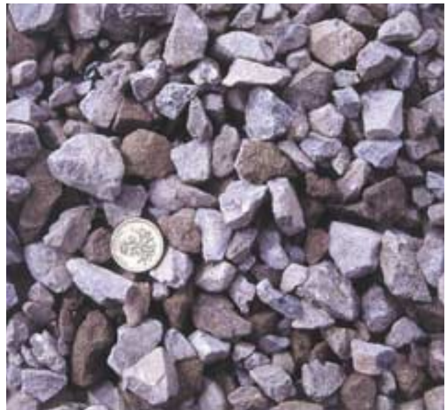
Pile of recycled concrete aggregate (RCA) – BS 8500 makes provision for the use of RCA.
