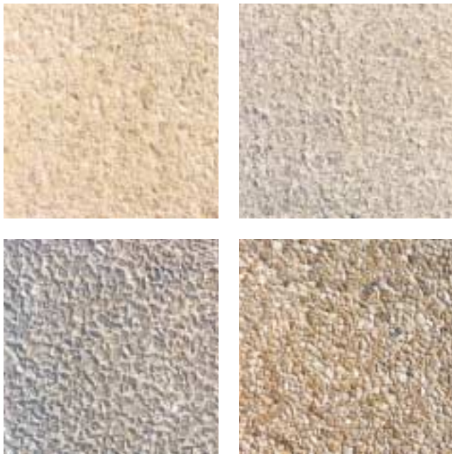
Four examples of exposed aggregate finishes – a special mix design is needed. Talk to your concrete producer. (Photo: CIL)
