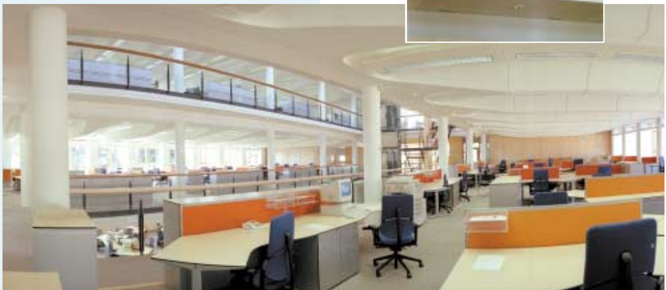
Canon UK offices, Reigate – Daylight is reflected by the concrete soffits, and the thermal mass of the concrete results in significant energy savings throughout the life of a building.
